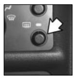
Press the button located under the air conditioning button to turn the defogger on. It will turn itself off after about 10 minutes. The rear window defogger uses a warming grid to remove fog from the rear window. It is designed to clear the center of the rear window first.
